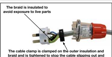
placing pressure on the individual conductors.
